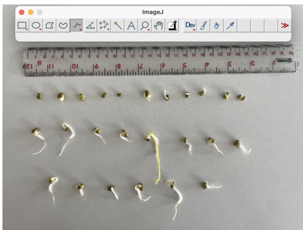
Figure 1. An Example of a Tracing on the Digital Analysis Program Used to Measure the Radicle Length
