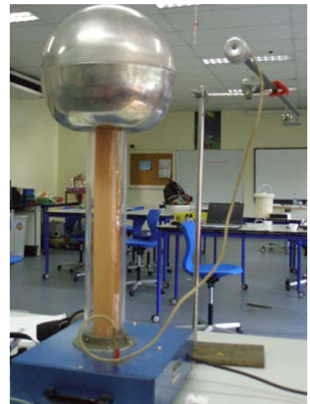
Figure 2: The wand was slowly moved towards the sphere until a spark sound (zap) could be heard.
