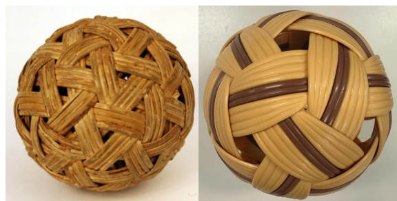
Figure 2. Traditional takraw ball made of rattan 2 (left) and the MT 201 Takraw ball used in this experiment (right).
