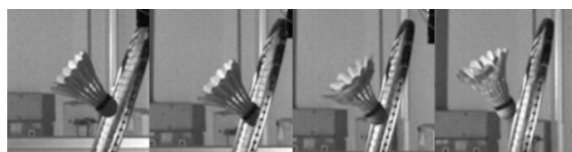
Figure 1. This series of images depicts the impact deformation of a Kason shuttlecock. 2
