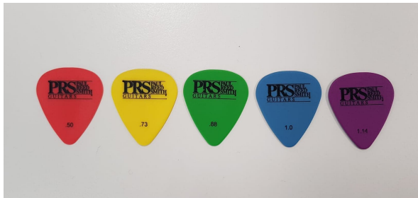
Figure 3. Top view of the picks of thicknesses from 0.50, 0.73, 0.88, 1.0 and 1.15mm. Picks are from Paul Reed Smith Guitars Delrin Touring Picks.
