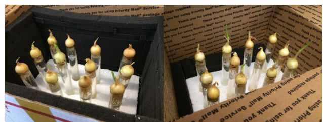
Figure 1. Sound chambers during root growth experiment: (left) sound stimulation chamber; (right) control chamber.
