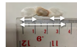
Figure 6 Measurement method for asymmetry (top) and total length (bottom).
